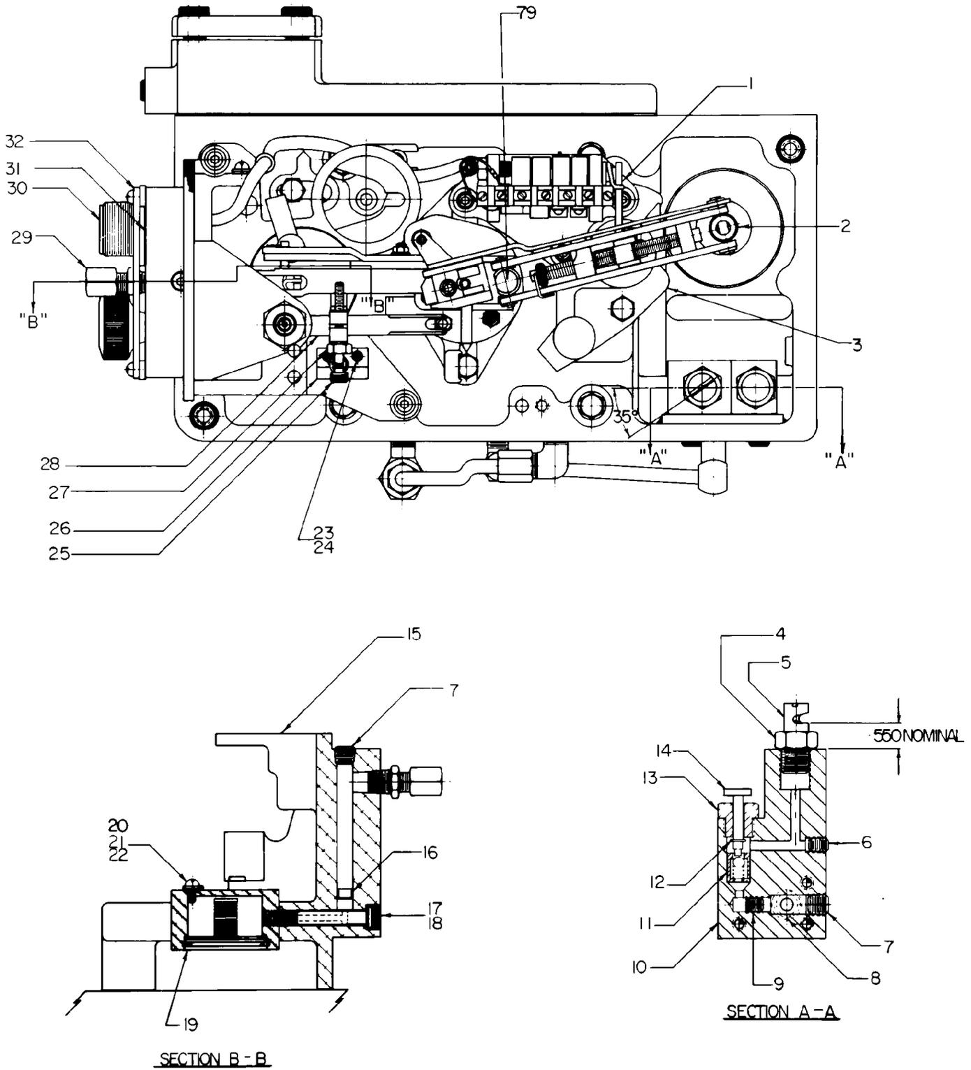
Figure 6. PGA-200 Vibration Resistant Governor with Oil Spray
