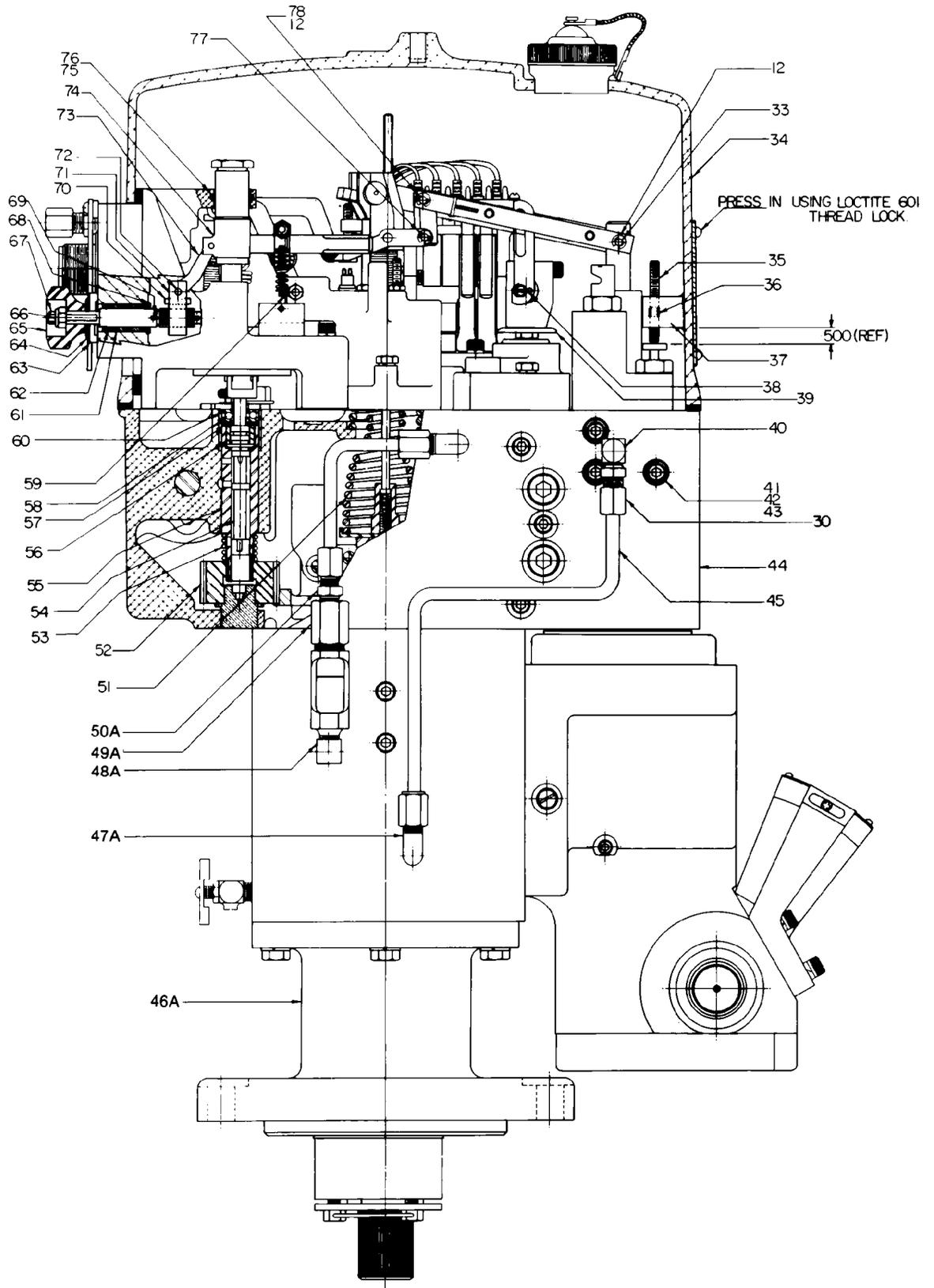
Figure 1. PGA-58 Vibration Resistant Governor with Oil Spray
