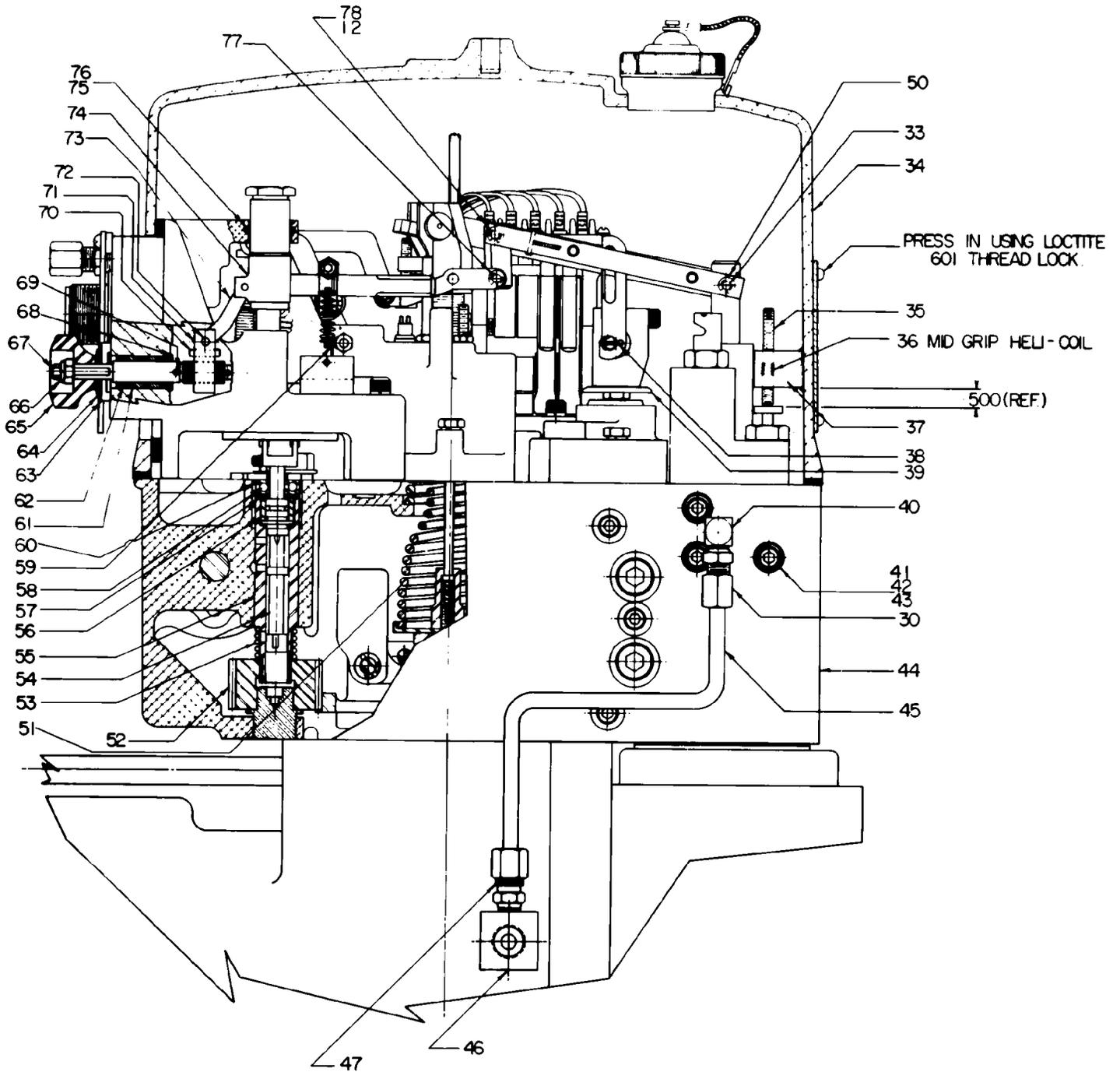
Figure 5. PGA-200 Vibration Resistant Governor with Oil Spray
