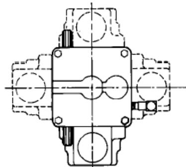
GOVERNOR CAN BE FURNISHED WITH SERVO MOTOR IN ANY OF FOUR PLANS AND QUADRANT POSITIONS AS SHOWN BY DOTTED OUTLINES.
